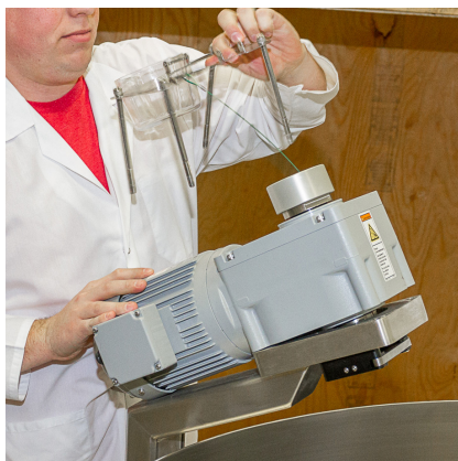
Figure 2.27. Placing the motor cap cover and bolts onto the motor and mount.
